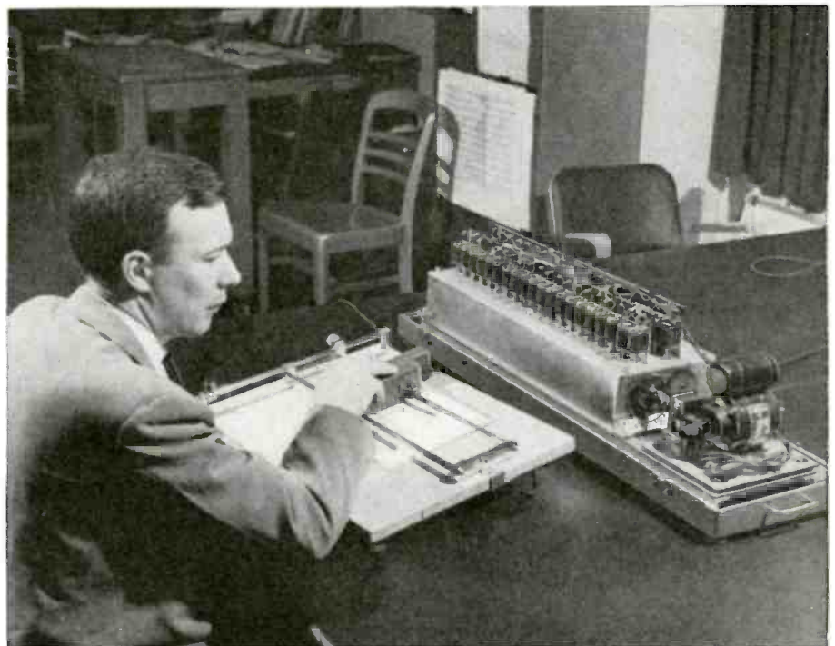
This device actually reads, pronouncing each letter as the phototube scanner moves over it.
